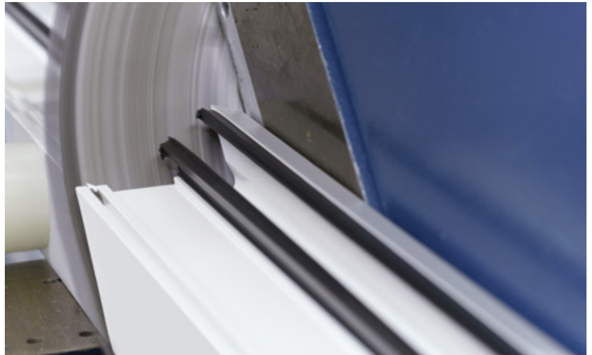
PVC-U profile preparation on machine technology with ionised air prevents swarf and dirt adhesion
